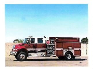
2008 International 4400 4X4, Pre-EmissionsDT570 (330HP), Allison 3000EV\_P Auto Transmission, Only 46,028 Miles, 2,728 Engine Hours, Pump and Drive, Block Heater, Fabco TC-237 2-Spd Transfer Case, 4.78 Rear End Ratio, 35,000 GVW, A/C, Crew Cab Seats 5 (4 SCBA Seats), Ferrara Fire Apparatus Body, Emergency Sirens and Intercom, Shelved Storage Compartments
